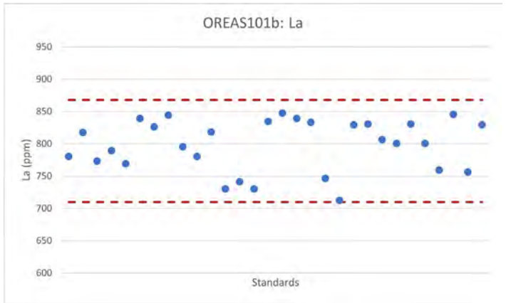
Figure 46 - Graphs of external CRM tolerances for Ce and La: OREAS-101b
