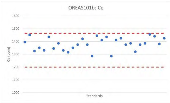
Figure 46 - Graphs of external CRM tolerances for Ce and La: OREAS-101b
