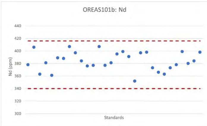
Figure 47 - Graphs of external CRM tolerances for Nd and Pr: OREAS-101b
