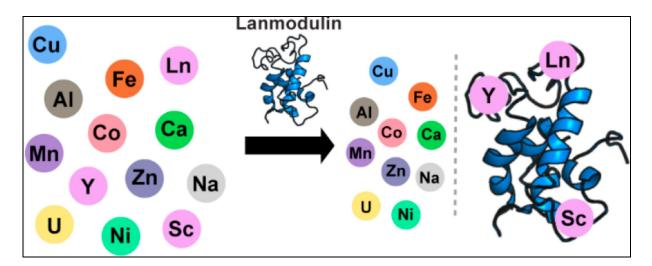
The schematic above seeks to show how the lanmodulin-based Rare Earth biosorption technology extracts the Lanthanides, Yttrium and Scandium. With this process high-purity Scandium and Lanthanides (Ln) can be produced from a single biosorption and desorption cycle, enabling selective Sc/Ln separation from other non-REE contaminants.
