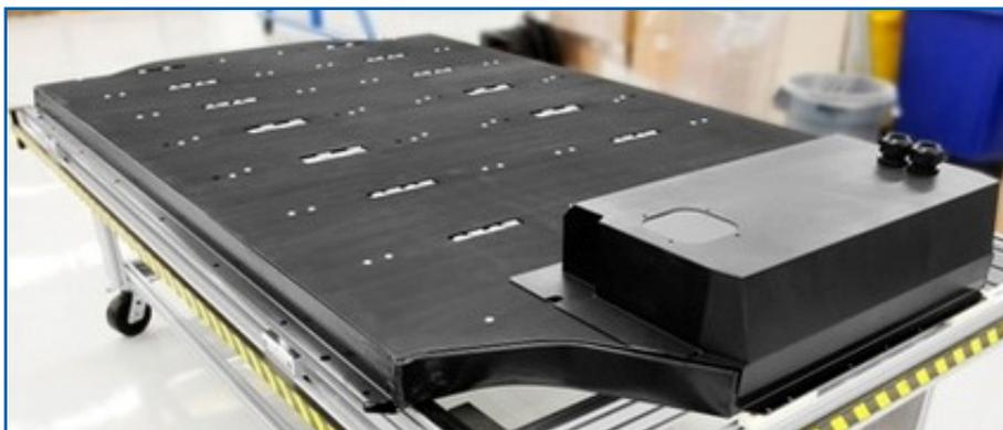
Tesla's Model S electric car's lithium cobalt battery pack
