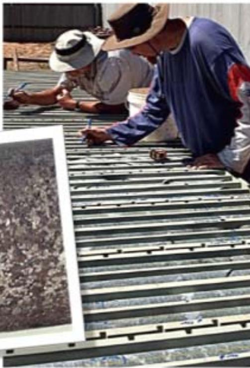
Figure 4. Marking up BED001 drill core with close-up (inset) of high-grade pyrite mineralisation.
